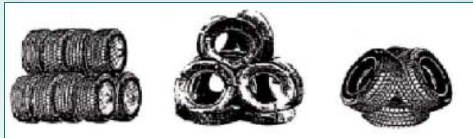
Figure 3.9 Poole Bay artificial reef tyre modules (courtesy K Collins, National Oceanographic Centre)
